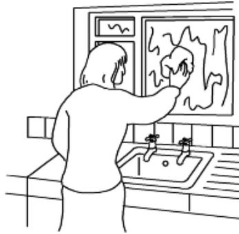
**Mould forms where condensation cannot dry out.** Your home needs fresh air as well as heat. Fresh air helps dry out surfaces.
